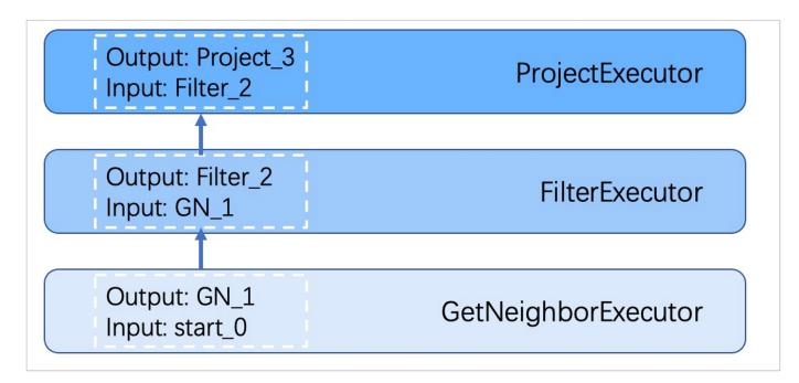
Each node of the execution plan has one execution operator node, whose input and output have been determined in the execution plan. Each operator only needs to get the values for the input variables, compute them, and finally put the results into the corresponding output variables. Therefore, it is only necessary to execute step by step from Start, and the result of the last operator is returned to the user as the final result.
