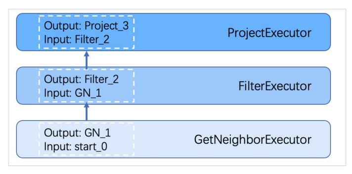
Each node of the execution plan has one execution operator node, whose input and output have been determined in the execution plan. Each operator only needs to get the values for the input variables, compute them, and finally put the results into the corresponding output variables. Therefore, it is only necessary to execute step by step from <code>Start</code>, and the result of the last operator is returned to the user as the final result.
