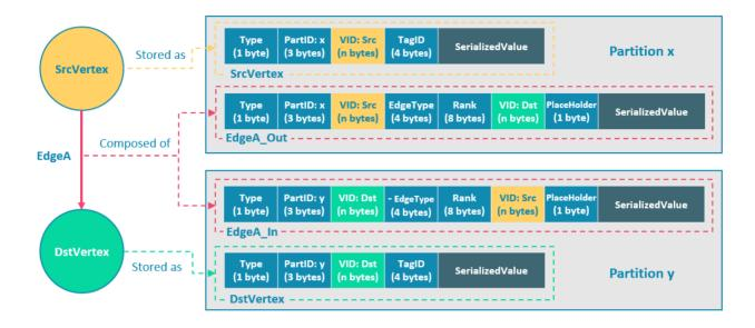
In this example, ScrVertex connects DstVertex via EdgeA, forming the path of (SrcVertex)-[EdgeA]->(DstVertex) . ScrVertex, DstVertex, and EdgeA will all be stored in Partition x and Partition y as four key-value pairs in the storage layer. Details are as follows:
