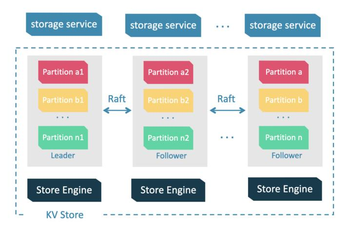
Storage Service is run by the nebula-storaged process. Users can deploy nebula-storaged processes on different occasions. For example, users can deploy 1 nebula-storaged process in a test environment and deploy 3 nebula-storaged processes in a production environment.
